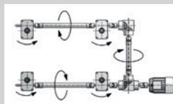
$$M_R = M_G \times 4,9 = 5,63 \text{ Nm} \times 4,9 = 27,59 \text{ Nm}$$
